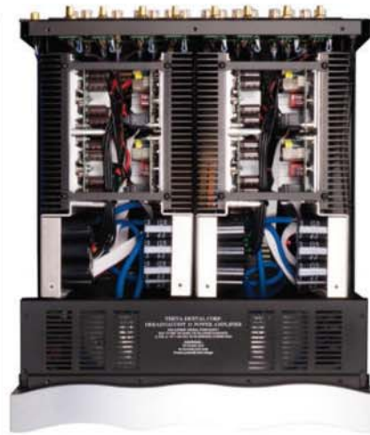
Dreadnaught class: inside Theta Digital's multichannel amp.
