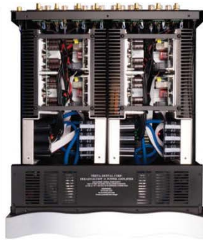
Dreadnaught class: inside Theta Digital's multichannel amp.
